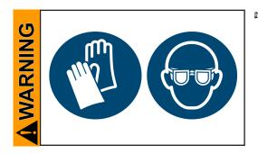
Use appropriate protective clothing, safety goggles and protective gloves. Take adequate precautions to protect people from the effects of dangerous substances that may have contaminated the pump and may be released upon disassembly. Ensure that the maintenance technician is familiar with the
