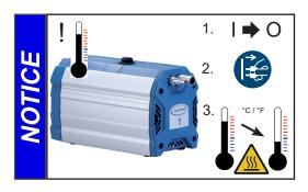
In case of overload, the motor is shut down by a **self-hold thermal cutout** in the winding. **Note**: Only manual reset is possible. Switch off the pump and disconnect from the power source. Identify and eliminate the cause of failure. Allow the pump to cool down sufficiently before restart
