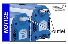
Outlet via hose nozzle for tubing I.D. 3/8" (hose nozzle DN 10 mm) (ME 1C, MZ 1C) or via silencer (ME 1).
