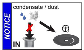
Prevent internal condensation, transfer of liquids or dust. The diaphragms and valves will be damaged, if liquids are pumped in significant amounts.
